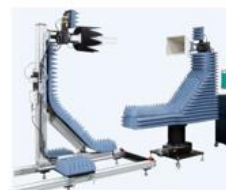
Antenna positioning and control system (0.5-20GHz, Antenna Size : Dia. 0.7m, Up to 18Kg,
