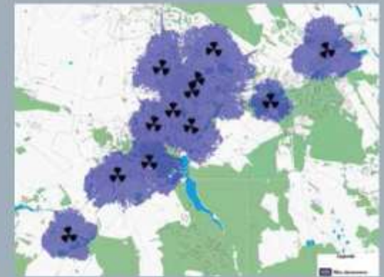
FIG. 1 MAP EXAMPLE OF HOW SAME/ LARGER AREAS CAN BE COVERED WITH A SMALLER NUMBER OF BASE STATIONS WITH EC RECOMMENDED EMF EXPOSURE LIMITS (RED) VERSUS RESTRICTIVE LIMITS (PURPLE)
